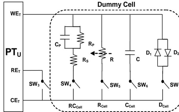
Fig. 5. Dummy cell and its connection to the  $PT_U$  ( $PT_U$ - potentiostat unit; SW- analog switch;  $RC_{Cell}$ - Randle's circuit cell;  $R_{Cell}$ - pure resistive cell;  $C_{Cell}$ - pure capacitive cell and  $RD_{Cell}$ - diode cell).
