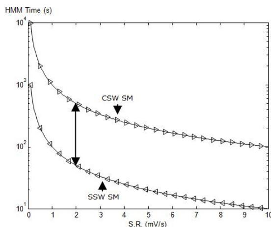
Fig. 4. HMM time for SSW and CSW sweeping modes (ratio between the sum of voltage sweep amplitudes and the voltage sweep range equal to 0.1,  $\Delta V_{CW}=5\text{mV}$  and a sweep voltage range amplitude equal to 1 V).
