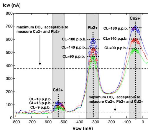
Fig. 12. Voltammograms of the water samples used for testing purposes (dotted line– CSW SM; circles – SSW SM for the low tide condition , triangles - SSW SM for the rising tide condition, diamonds - SSW SM for the high tide condition).
