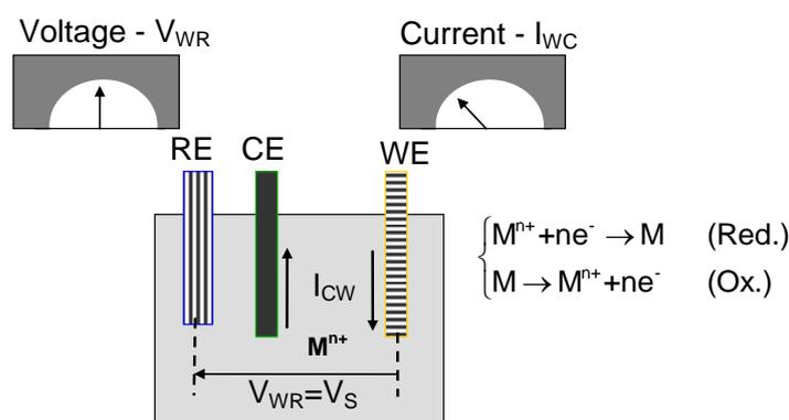
Fig. 1. Three electrodes measuring cell (WE- working electrode; CE- counter electrode; RE- reference electrode;  $I_{CW}$ - current between working and counter electrodes;  $V_{WR}$ - voltage between working and reference electrodes;  $V_S$ - source voltage; Ox.- chemical oxidation equation; Red.- chemical reduction equation;  $M^{n+}$ - dissolved ion).
