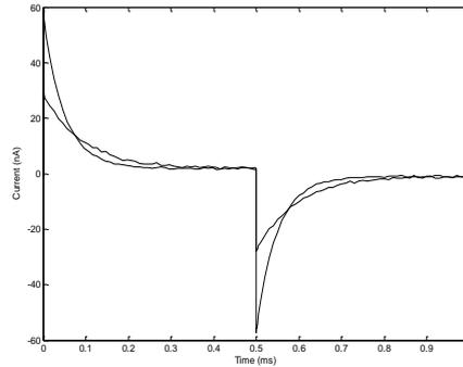
Fig. 6. Voltage-to-current characteristic of the  $RC_{Cell}$  for the following set of parameters:  $R_S=2\text{ M}\Omega$  (upper curve),  $R_S=4\text{ M}\Omega$  (lower curve),  $R_P=20\text{ M}\Omega$  and  $C_P=30\text{ pF}$ .
